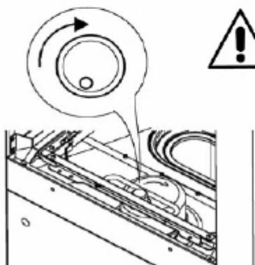
**WARNING:** In case of wrong direction of rotation, the mechanical to ensure the shift is ineffective.
